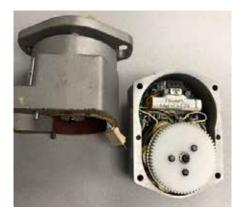
Remove hardware holding the driven gear/magnet arm assembly. Pull driven gear/magnet-arm assembly, from the driven shaft.
