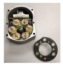
Remove three screws and lock washers. Then pull the entire pickup plate assembly off bearing.
