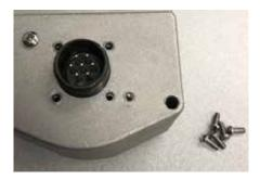
From outside of unit install connector mounting screws and heatsink mounting screw.
