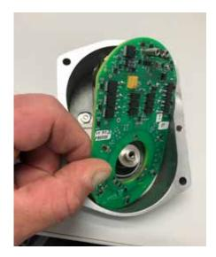
Fasten circuit board assembly to casting using hardware provided, only three screws will align with the tapped holes in machined back cover.
