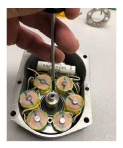
Location of pickup assembly mounting screws.
