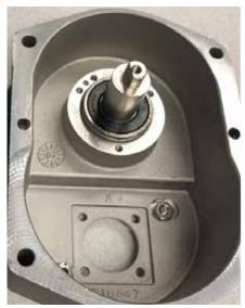
Hole plug screw assembly installed in the location of old Zener.
