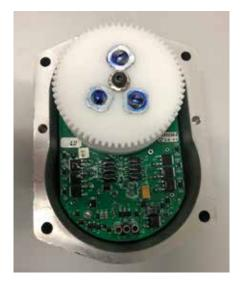
Alternator update is done next. The existing magnet Rotor assembly will be replaced with a new, more powerful, rare earth magnet assembly.
